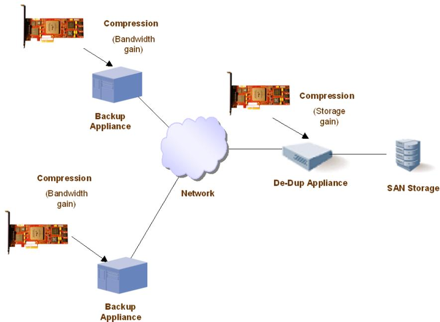
**Figure 1: Compression Accelerator boards in Network Appliances**
