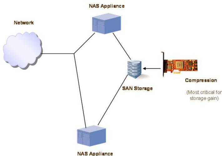
**Figure 2: Acceleration board in a Storage Attached Network (SAN) Appliance**
